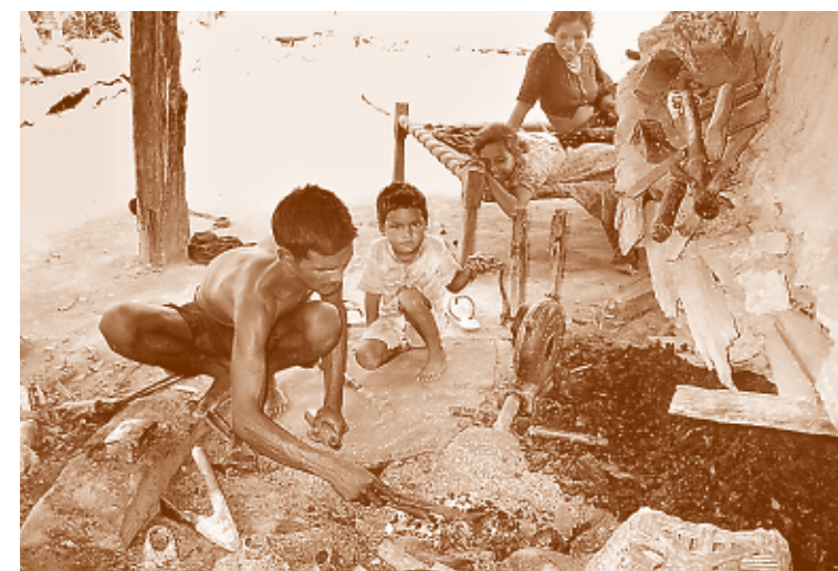
A Bishwokarma man metal working, helped by his son turning the bellows.
